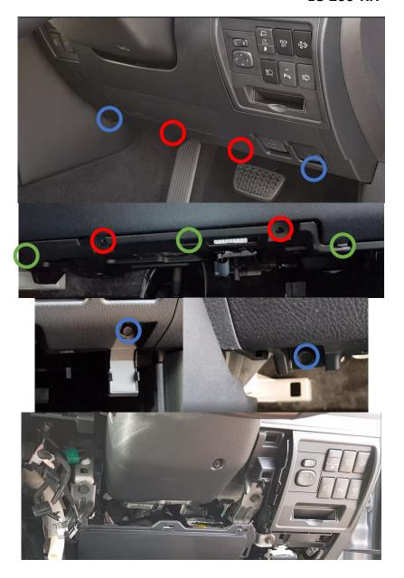
There is a total of 4 screws to remove in this install.
